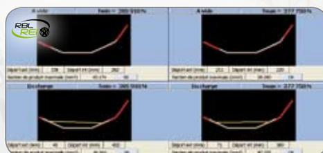
Regardless of the number of bends and the convex and concave shape of the conveyor belt, this calculation means that the very best design can be chosen ensuring a the stable performance of the belt in all operating stages, such as
